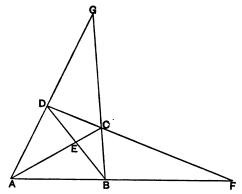
Let A, B, C, D be any four points, and let the connectors AC, BD meet in E, the connectors AB, CD in F, and the connectors AD, BC in G. Then E, F, G are the centres of the tetrastigm ABCD.
